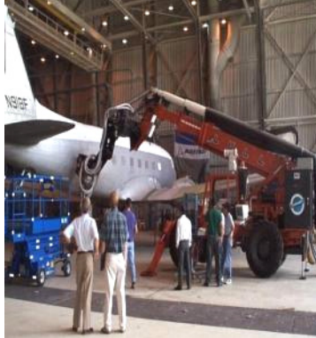
FLASHJET® deployed using commercial rough terrain fork lift with servo pivot and boom.
