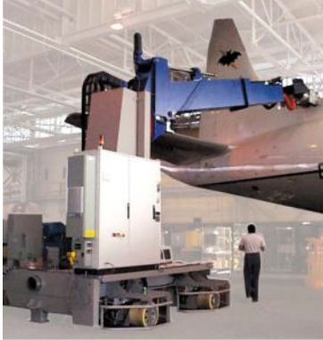
Full FLASHJET® system with omni-directional vehicle deployed on forward rudder.
