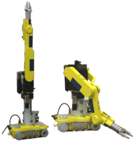
Robot range of reach is 3.5 m (11 ft. 5 in.) to floor level.
