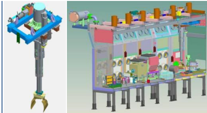
PaR is working on the PDCF Pit Disassembly and Conversion Facility (PDCF) at Savannah River Site. This system requires multiple telescoping tubes to create a profile that is very compact to work inside a glove box with Argon and Helium atmosphere. The robot is designed for installation and removal through small “bag out” ports with circular openings.
