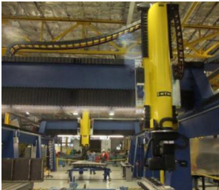
Dual-Bridge Gantry System
