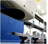
an adaptive tool path that corresponds with the current contour. The part is cut in the unconstrained state in such a way that it will be the correct size when it is constrained to its nominal shape when installed in the aircraft.
