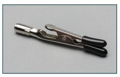
Load Cell Specimen Holder (Clip type)
